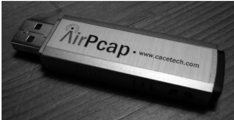
Figure 10-3: The AirPcap device is very compact, making it easy to tote along with a laptop.
