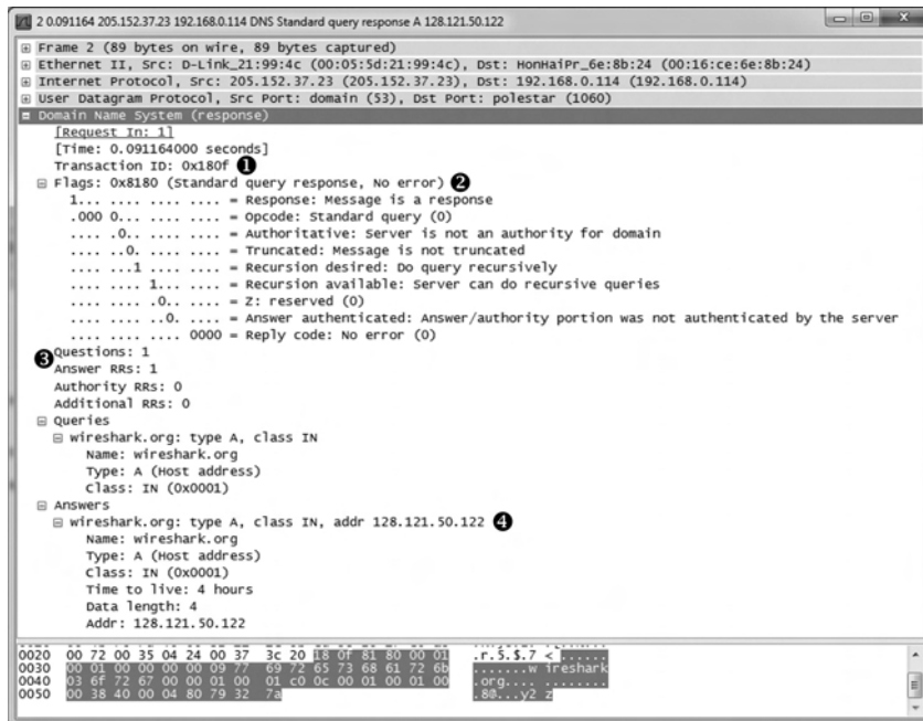
Figure 7-9: The DNS response packet
