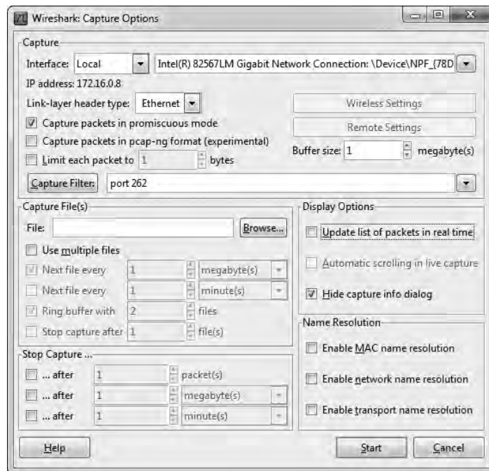
Figure 4-10: Creating a capture filter in the Capture Options dialog
