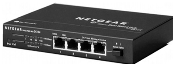
Figure 1-4: A typical 4-port Ethernet hub
