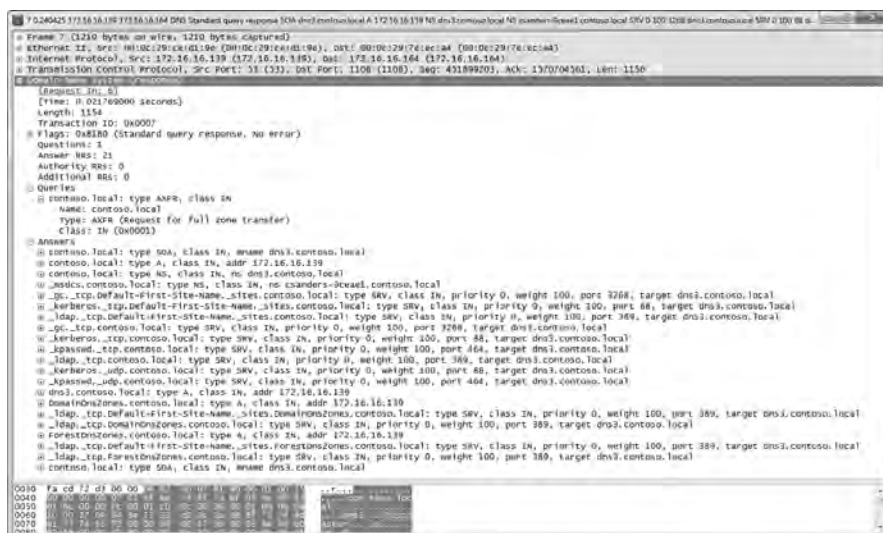
Figure 7-17: The DNS full zone transfer occurring
